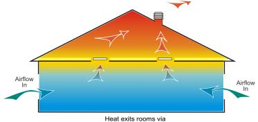
Heat exits rooms via ceiling registers into roof area and out Condor Roof Ventilator
