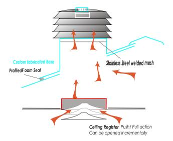
Ceiling registers are manually opened using a claw on the end of a suitable length of rod The push/pull mechanism, opens and closes on demand using rod and claw. This allows for efficient heat purging of during summer evenings and prevents heat loss during winter months.
